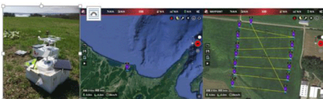
Figure 2: UAV with multispectral camera (Left), Observatory eastern part of Hokkaido (Middle) and Pre calculated course on grass land (Right).
